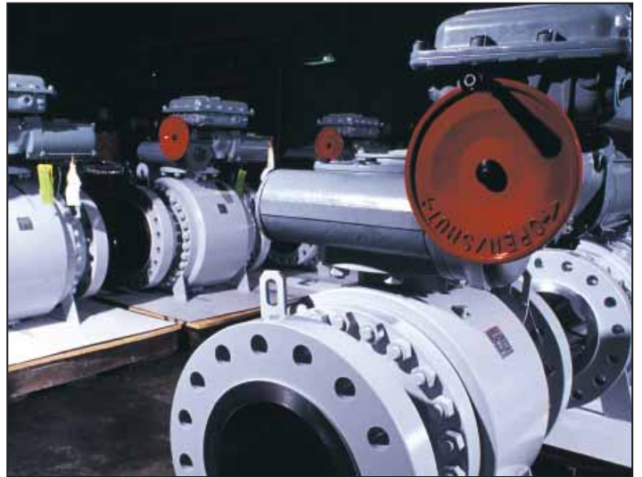
The valves shown above are just a few of many severe service ball valves PBV® produced for the United States Department of Energy, Strategic Petroleum Reserves, complete with gear operators built and tested to DOE specifications.
