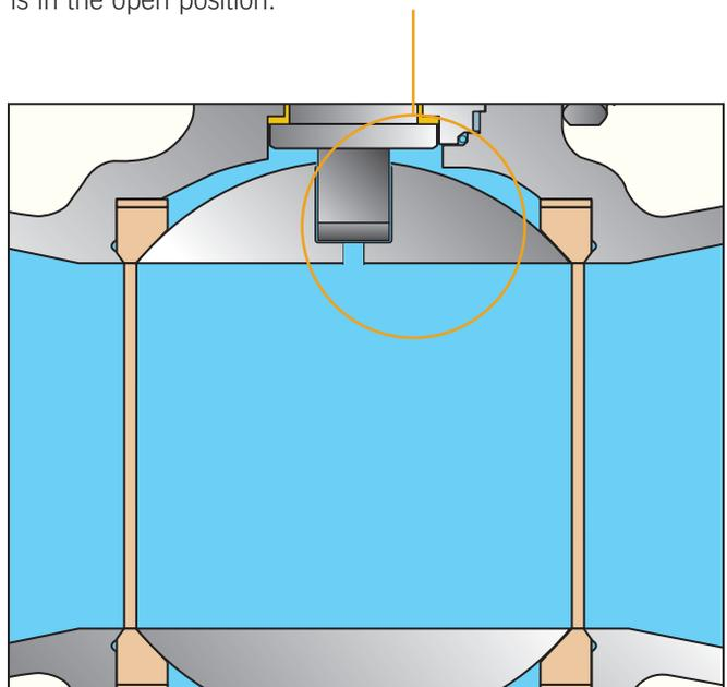
PBV® Valve's Series 4400/6400/5400/4500/6500 valves have all been proven to be Firesafe to API 607 or API 6FA. As illustrated, full metal-to-metal contact is attained at all sealing areas after the primary soft seals have been destroyed during a fire.
