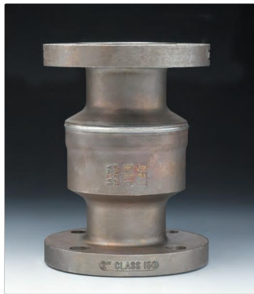
The **DFT® Model DLC Check Valve** is a corrosion-resistant, dependable, versatile and economical spring assisted, non-slam check valve for a wide range of applications. Whether the fluid is liquid, gas or steam, the DLC check valve provides tight shutoff and protects other equipment in the system from water hammer. Its stainless steel construction insures a long service life.
