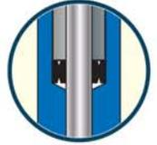
**3** Special double V-shape of stem seal self-adjusts to protect the stem area for either vacuum or pressure use.
